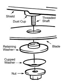
**NOTE:** Make sure all parts are in place as illustrated, and the blade is sandwiched between the dust cup and the retaining washer. There should be no space between the blade and the dust cup or the retaining washer.
